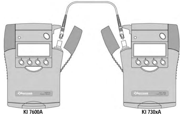
Test set-up for the Output Power Test
