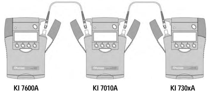
Test set-up for the Power Meter Accuracy Test
