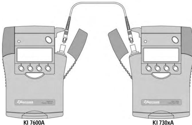
Test set-up for the Short Term Stability Test
