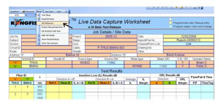
14. Now you have set up your test. With the meter still in Autotest mode, click on a Ref A or Meas B cell (yellow background), and you will get reference A values and Measurement B values entered for all wavelengths of the selected fiber. The other cells (in light blue colour which indicates system output) are filled in automatically. 15. Go ahead, fill some more values, and see how quickly you can work like this.
