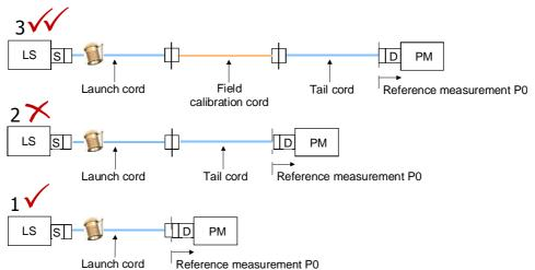
Enter the allowed test cord referencing configurations, separated by a comma. Thus to permit all 3 configurations use 1,2,3. For 1 & 3 lead referencing only enter 1, 3.
